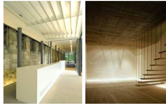
Concealed uplighting and lighting of vertical surfaces
