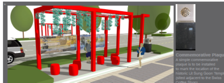
Pergola structure (west) seen from footpath Pergola Structures Model of the proposed steel pergola structures (2.6m x 8.6m x 3.7m high). These simple steel structures are based on traditional Chinese lattice work. The steel is finished in a high gloss red to reflect the Chinese love of this auspicious colour.
