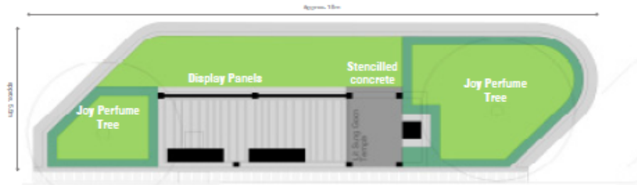
Plan of proposed Chinese microsite - site of the historic Lit Sun Goon Temple (no 95 Grafton St) Shows layout of microsite showing the footpath treatments (grey) planting (green) formal hedge (dark green). The pergola structure is outlined in black, with the temple commemorative plaque to far right of island, and two timber benches (black) island to be linked to the footpath to provide continuity with the main pedestrian thoroughfare.
