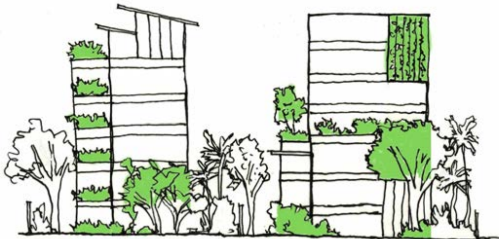
Figure SC6.16.3.7.b – Front elevation (Landscaping in green is used to calculate vertical landscaping coverage)
