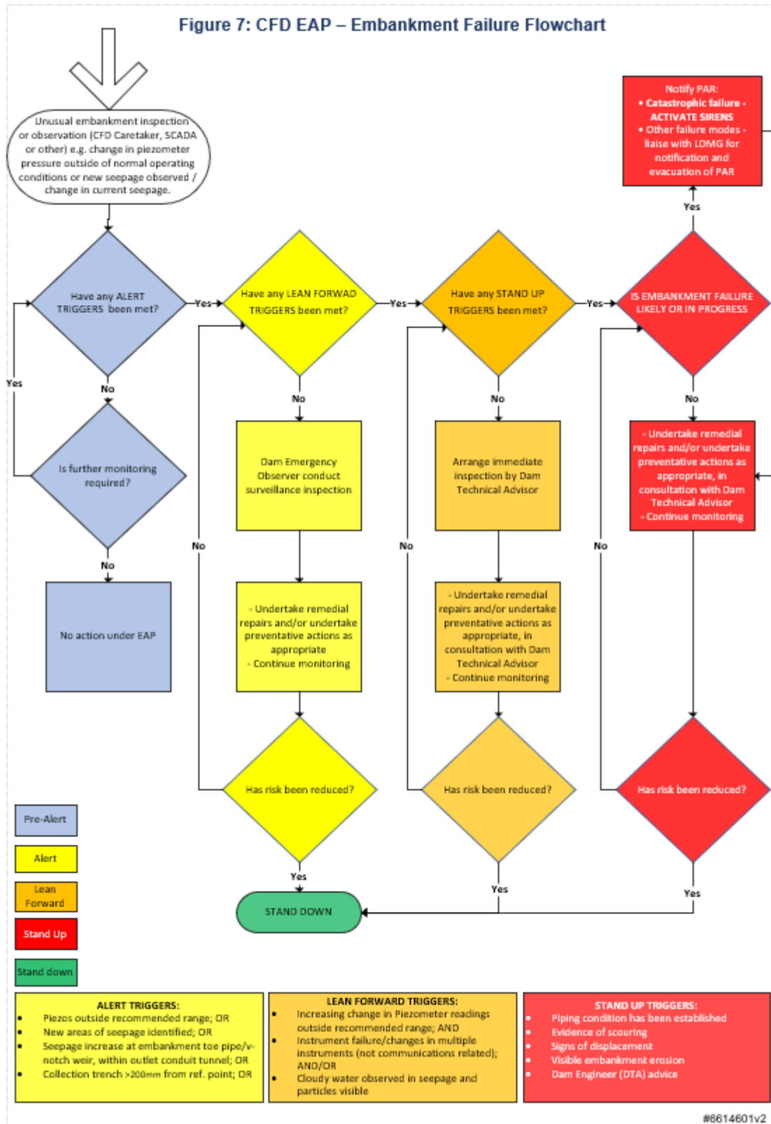
Figure 7: CFD EAP – Embankment Failure Flowchart
