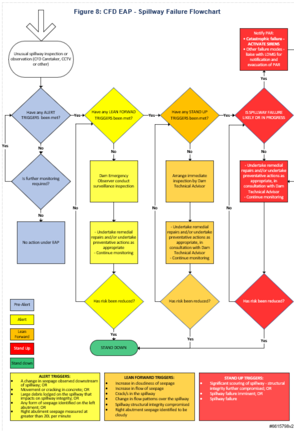
Figure 8: CFD EAP – Spillway Failure Flowchart
