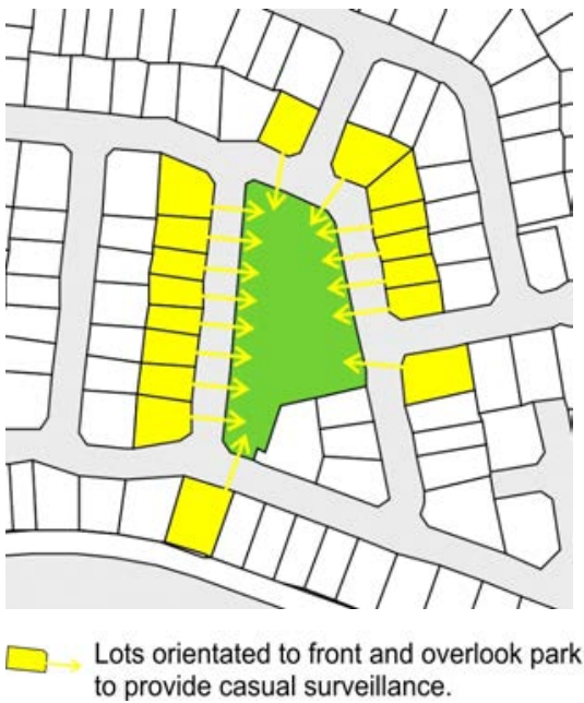
Figure 9.4.9.3.b – Consistent design solution for the orientation of lots surrounding open space and parkland
